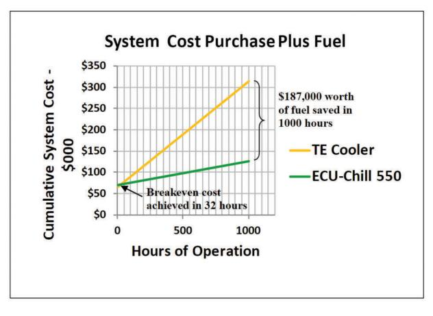
Figure 4 ECU-Chill provides significant energy cost savings in field operation.
