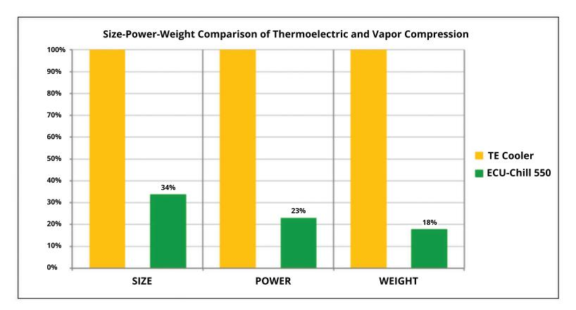
Figure 3 Vapor Compression cooling is 3 times lighter, 4 times more efficient, and 5 times lighter than thermoelectric
